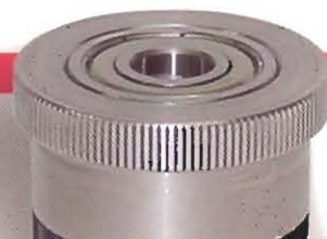
Saxon sealer pressure-wheel coarse knurl seal pattern
