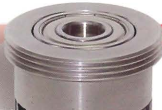
Saxon sealer pressure-wheel thread form seal pattern
